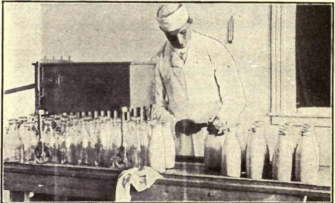
Fig. 62.—Filling Bottles with Machine. (From Da. Div., U. S. Dept. of A.)
